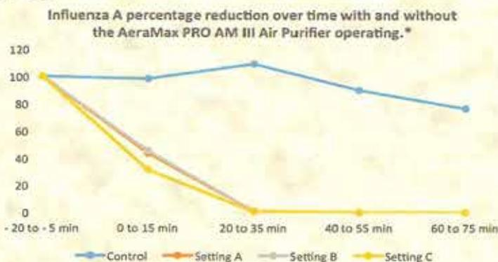
\*Results represent the average of n=3 runs. Device settings A: ionizer ON and filter low speed; device setting B: ionizer off and filter at low speed; device setting C: ionizer on and filter at high speed.
