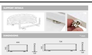
This open white painted aluminium frame support features an easy glide for the graphic poster (5mm max. thickness). Also, it features 2 magnetic supports at the bases. Ideal for promoting on shelves at malls or at the supermarkets.
