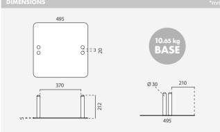
$The Balboa\,XL is\,made\,of\,steel\,sheet\,of\,5mm\,thickness. It features\,black\,laquered$ (RAL 9005) or grey laquered (RAL 9006) finish. This XL Steel base is ideal to hold rigid materials of 19mm thickness. Specially designed for supporting big graphic panels (2000mm max. height recommended) thanks to its 10.65kg.
